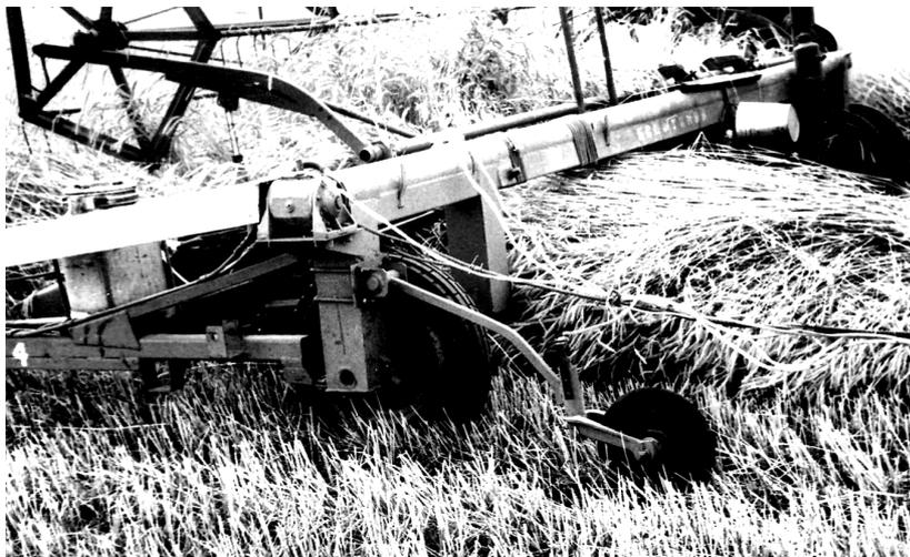
**Fig. 1. Base (factory) variant of setting left supporting wheel of trailed swath header ZVP-6 (behind the left supporting wheel of the swath header there is mounted a track measuring wheel)**
